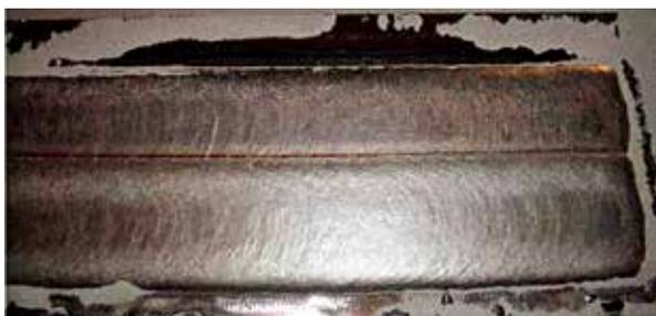
图79 昆山京群GDS-2209/GXS-S330双相不锈钢带极电渣焊
